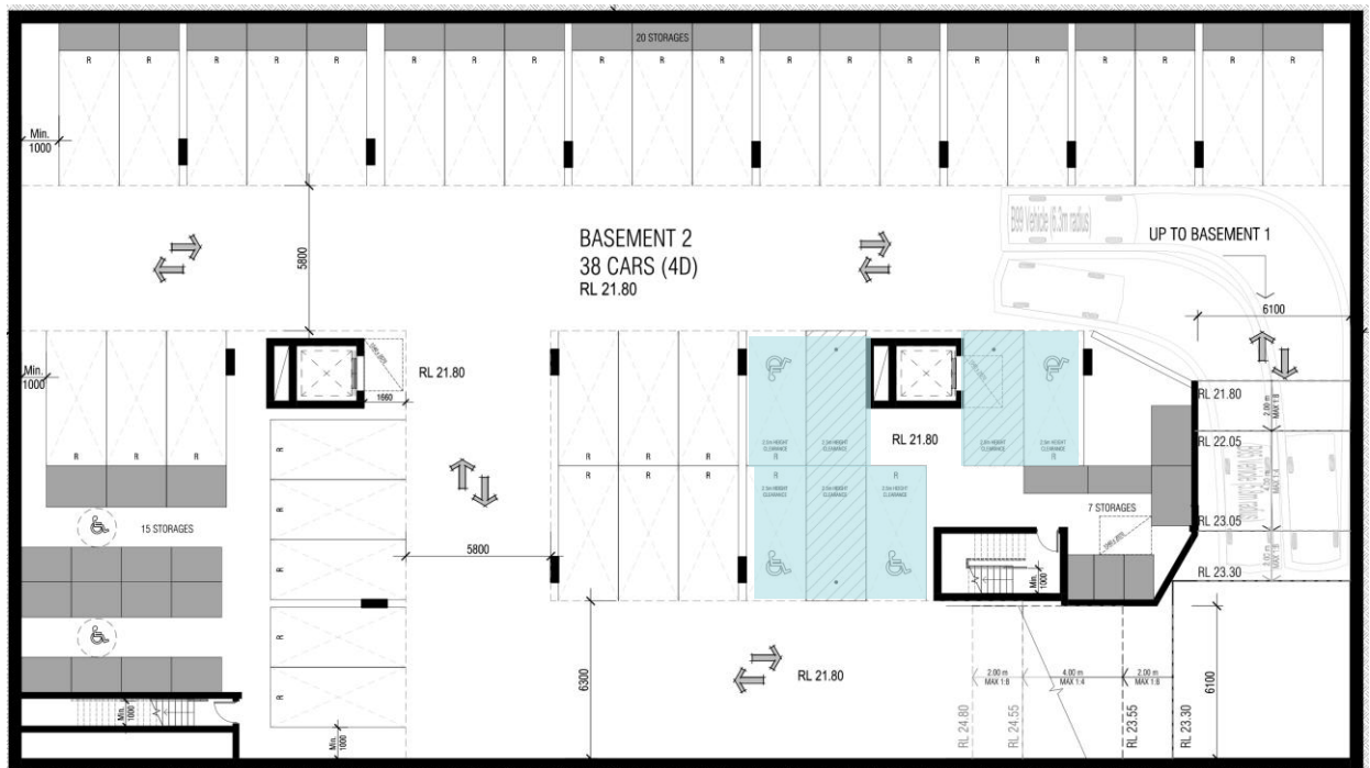
[Image description: Plan of Basement 2 levels above shows the provision of Accessible parking spaces]
